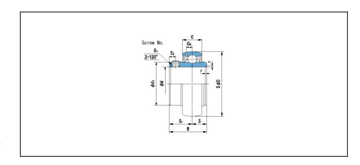
Basic Dynamic Load Rating Cr : 19600 N INNER RING OUTER RING
