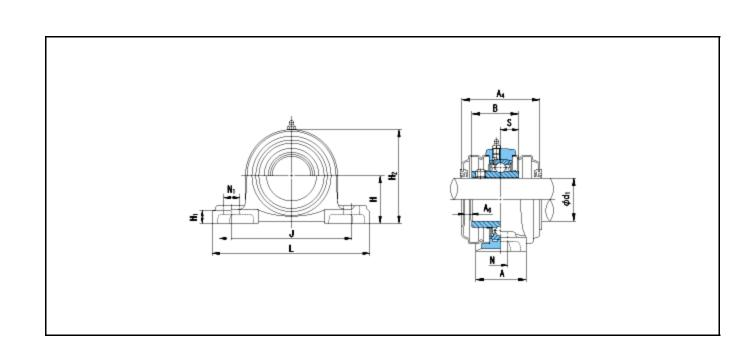
Basic Dynamic Load Rating Cr : 57500 N INNER RING OUTER RING
