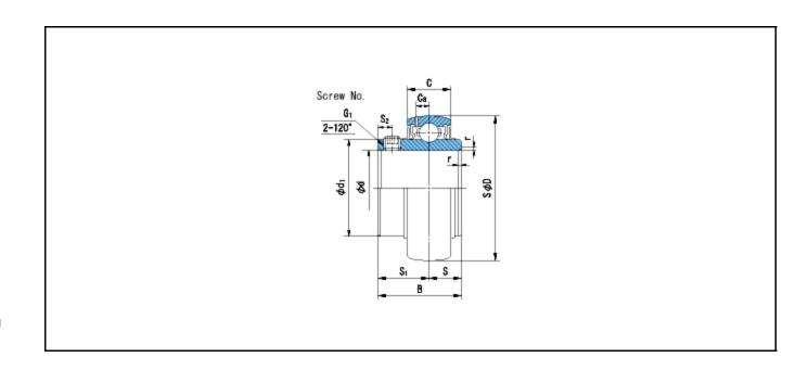
Basic Dynamic Load Rating Cr : 114000 N INNER RING OUTER RING
