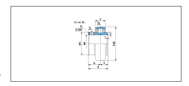
Basic Dynamic Load Rating Cr : 92500 N INNER RING OUTER RING
