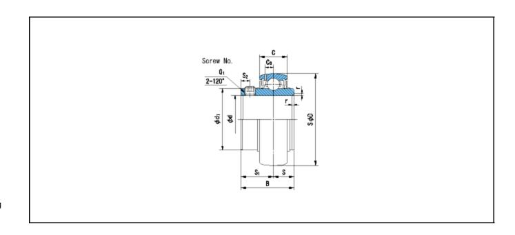
Basic Dynamic Load Rating Cr : 26800 N INNER RING OUTER RING
