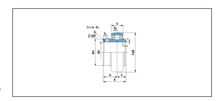
Basic Dynamic Load Rating Cr : 21300 N INNER RING OUTER RING
