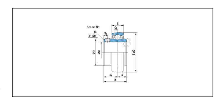
Basic Dynamic Load Rating Cr : 72500 N INNER RING OUTER RING
