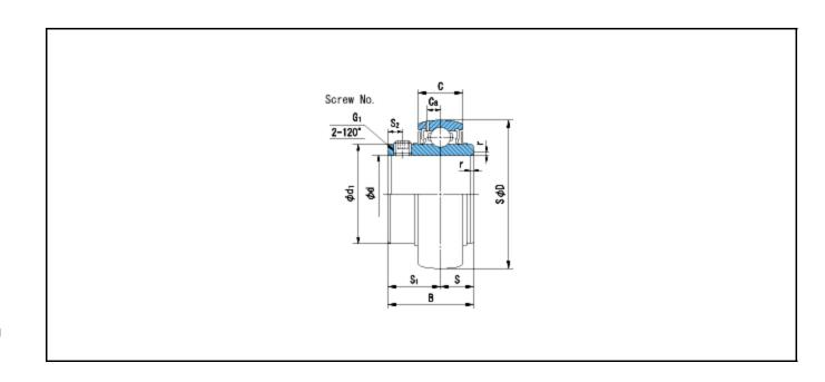
Basic Dynamic Load Rating Cr : 35500 N INNER RING OUTER RING
