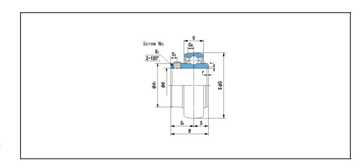
Basic Dynamic Load Rating Cr : 19600 N INNER RING OUTER RING
