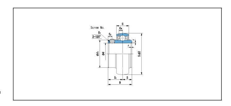
Basic Dynamic Load Rating Cr : 12800 N INNER RING OUTER RING
