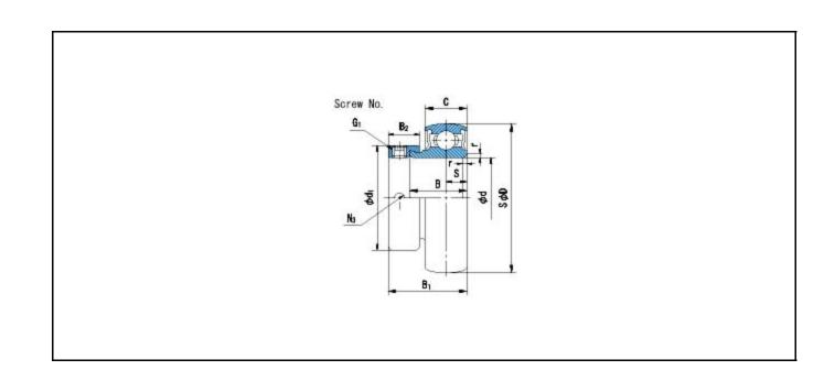
Basic Dynamic Load Rating Cr : 3300 N INNER RING OUTER RING
