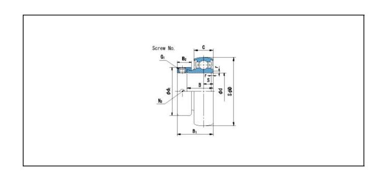
Basic Dynamic Load Rating Cr : 5100 N INNER RING OUTER RING
