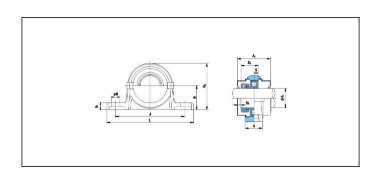
Basic Dynamic Load Rating Cr : 8600 N INNER RING OUTER RING
