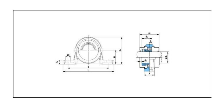
Basic Dynamic Load Rating Cr : 7900 N INNER RING OUTER RING
