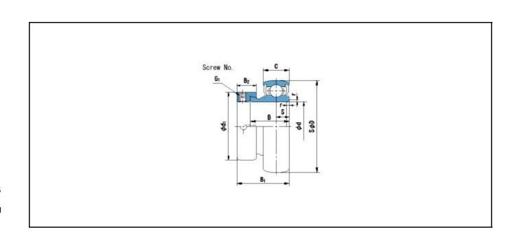
Basic Dynamic Load Rating Cr : 25900 N INNER RING OUTER RING
