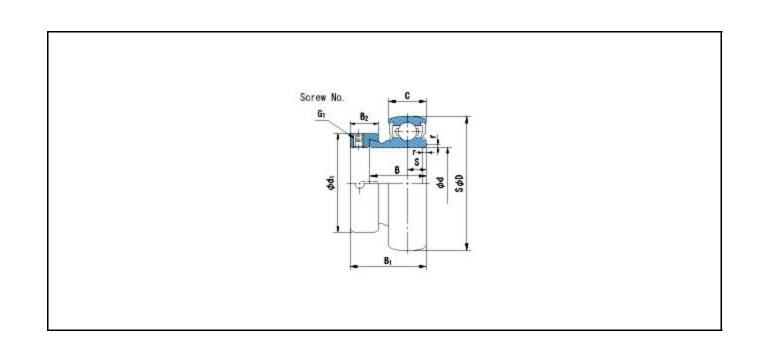
Basic Dynamic Load Rating Cr : 14000 N INNER RING OUTER RING
