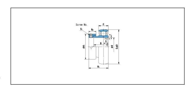
Basic Dynamic Load Rating Cr : 9550 N INNER RING OUTER RING
