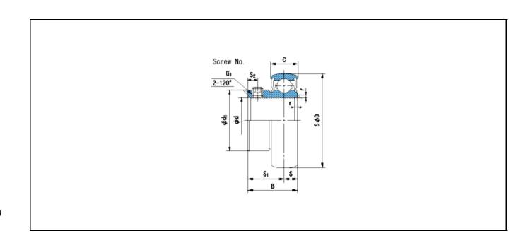
Basic Dynamic Load Rating Cr : 25900 N INNER RING OUTER RING
