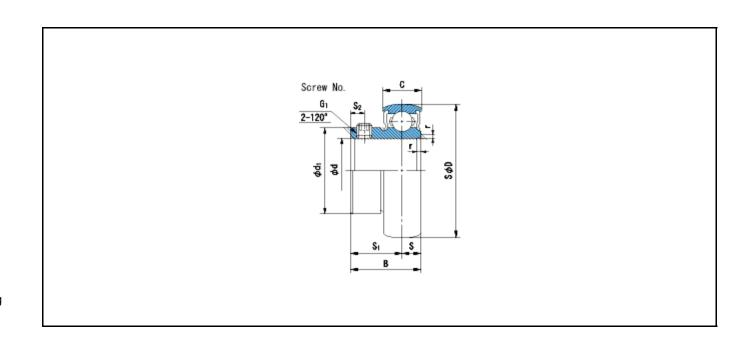
Basic Dynamic Load Rating Cr : 14000 N INNER RING OUTER RING
