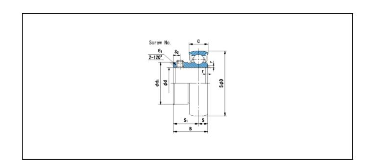
Basic Dynamic Load Rating Cr : 9550 N INNER RING OUTER RING
